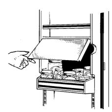
The Countermaker Compartment is also accessible through a lift-up door on the inside of the fresh food compartment door.
